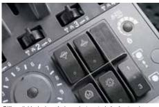
Differential locks have independent controls for front and rear axles.
